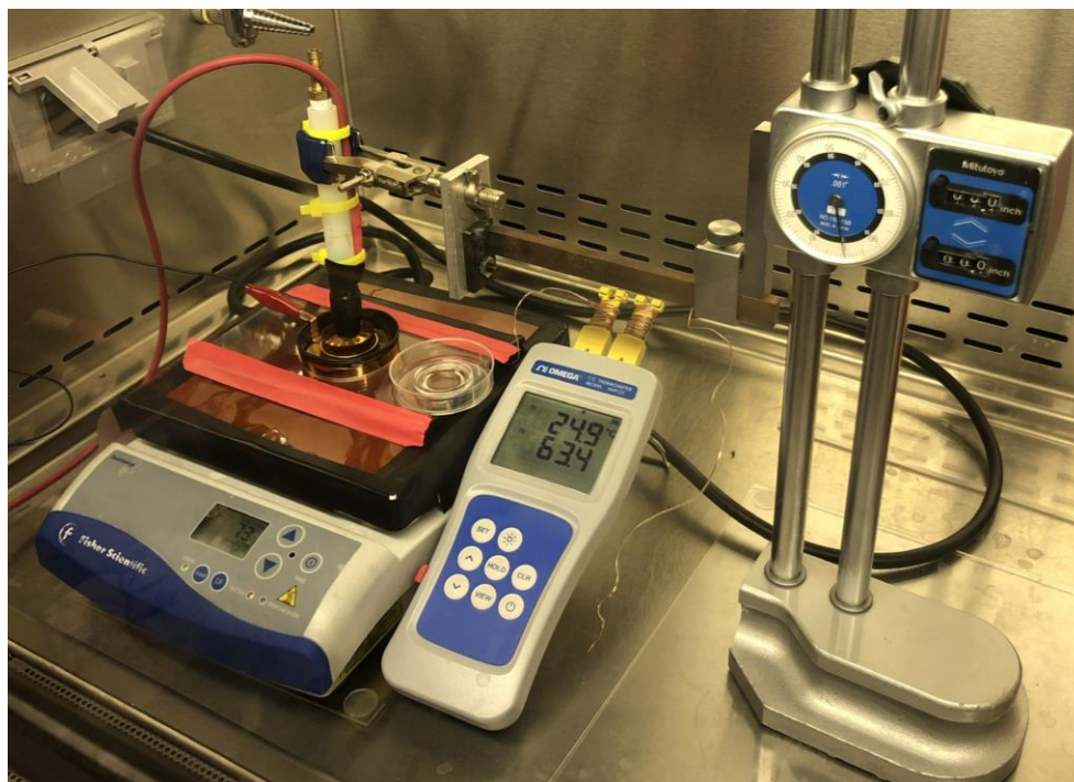
Figure 3.10: Hot plate set up. The thermocouple on the left connects to the metal plate while the thermocouple on the right would be used in the cell solution until corona was applied.
